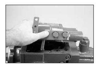
**Step 4**Remove the control valve gasket from the pump housing and discard.
