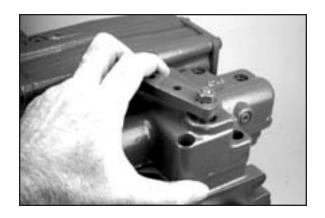
**Step 4**Remove and discard the control valve gasket.
