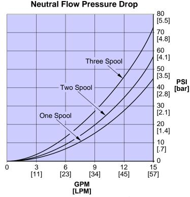
Test performed with oil viscosity 150 SUS @ 100° F [37.7° C] – oil temperature 130° F [54.4° C]
