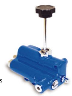
Similar to other single spool control valves, this valve allows the operator to smoothly position (raise and lower) the mower deck or reels with precision. In addition, lift circuit back pressure can be modulated by operating a rotary needle cartridge which allows the operator to take weight off the cutting units for reduced ground pressure and increased tractive effort or to apply down pressure to the cutting units for improved cutting finish.
