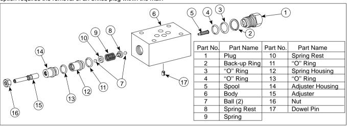
Figure 10. Reducer Module
