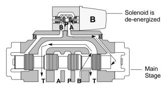
The spring returns pilot spool to "A" offset position and shifts main stage spool. Main stage oil flow is  $P \rightarrow A$  and  $B \rightarrow T$ .
