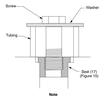
Thread seat (17), then place tubing and washer over seat area as shown. Thread the screw into seat. Tighten the screw to remove seat.
