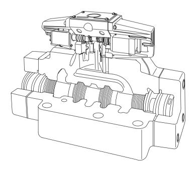
Figure 2. Typical 'DG5' Type Solenoid Controlled, Pilot Operated Valve
