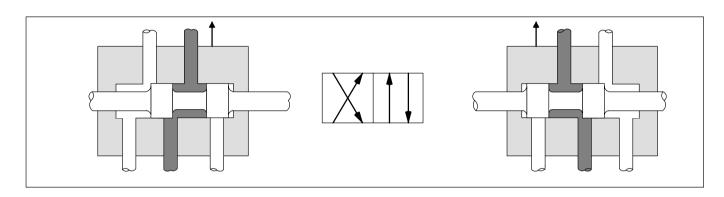
Figure 1. Spool Type Four-Way Valve
