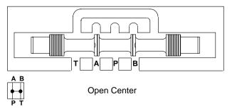
B. Type '1' spool is designed with ports (P), (A) and (T) interconnected. Port (B) is blocked in center position.
