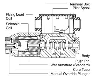
Figure 13a. Typical DG4V-3(S)-A/B-FW-60
