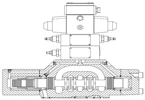
Figure 11. DG5V10 with DG4S4-01 Pilot
