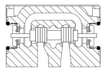
Figure 12c. Flow Conditions Flow Blocked (Center Condition #2 Spool)
