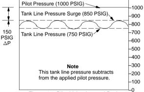
Figure 14. Pilot Valve-Internal Drain
