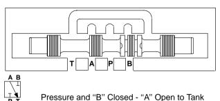
C. Type '6' spool is interconnected at ports (A), (B) and (T). Port (P) is blocked in the center position.
