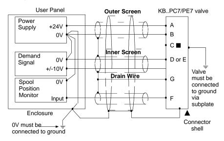
■ Spool position monitor voltage (pin F) will be referenced to the KB valve local ground. A "local ground" (pin C) is provided on PC7/PE7 versions for optional use by differential input customer supplied electronics.
