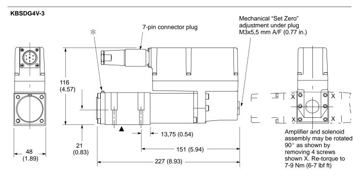
▲ Mounting surface seals supplied. For mounting surface dimensions and subplate options see page 9.
