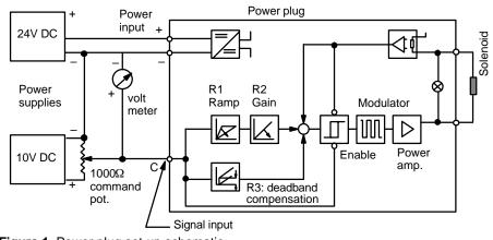
Figure 1. Power plug set-up schematic
