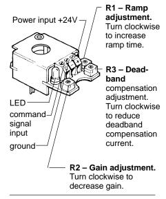
Figure 2. Power plug connections
