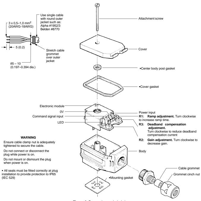
Figure 6. Power plug exploded view
