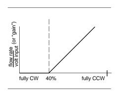
**Figure 4.** Sensitivity of deadband adjustment to potentiometer R3 (typical).
