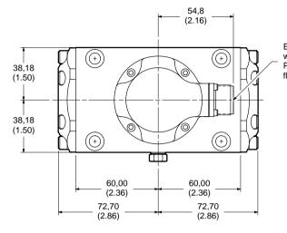
Electrical connector mates with MS-3106-14S-2S (4 pin). Plus signal to A or C causes flow out of port B.
