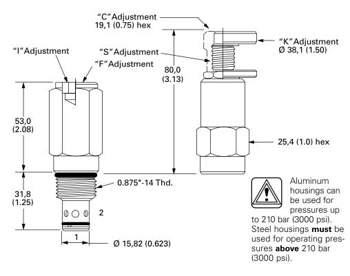
Thermal relief with reverse flow check valve
