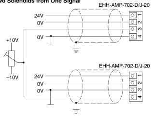
Connections when replacing –10 design power plug with –20 design and only 3 wires exist
