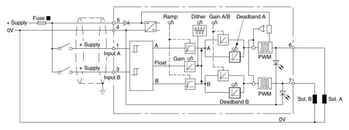
Note: Models E and F operate the "A" solenoid only. The "B" channel components are not fitted.
