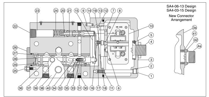
Figure 6. Servo Valve Assembly - Cross Sectional View
