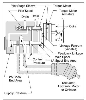
Figure 1. Servo Valve Schematic
