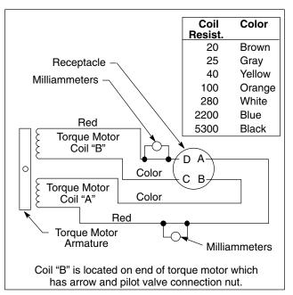
Figure 4. Wiring Diagram – Schematic View
