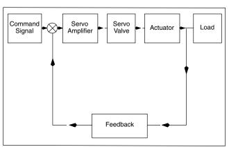
Figure 2. Servo Valve System Block Diagram
