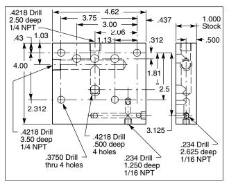
Figure 3. Flushing Plate (938714)
