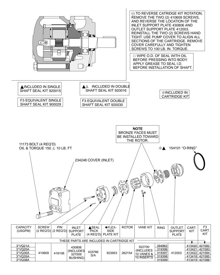
○ ASSEMBLE SEAL WITH SPRING LOADED SEALING MEMBER TOWARD BEARING.
