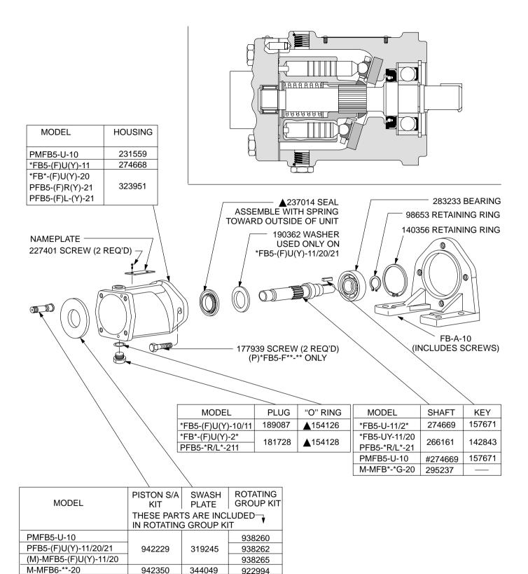
▲INCLUDED IN 919239 SEAL KIT F3 EQUIVALENT SEAL KIT 919311 #WHEN ORDERING THIS SHAFT, ALSO ORDER 273409 LIFT LIMITER.
