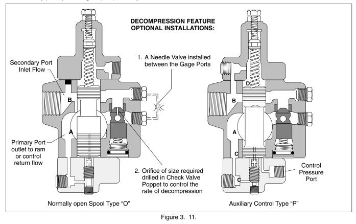
Valves with the "P" feature, auxiliary remote control are available in both the R\* and the RC\* series.
