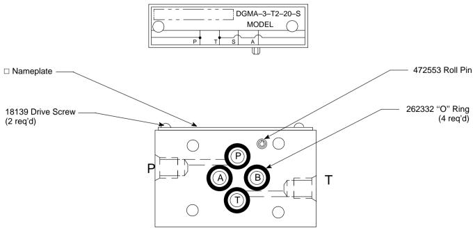
□ Name Plate read from 'P' port side with "O" ring grooves downward.
