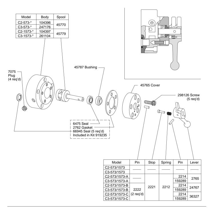
For satisfactory service life of these components, use full flow filtration to provide fluid which meets ISO cleanliness code 20/18/15 or cleaner. Selections from Vickers OFP, OFR and OFRS filter series are recommended.
