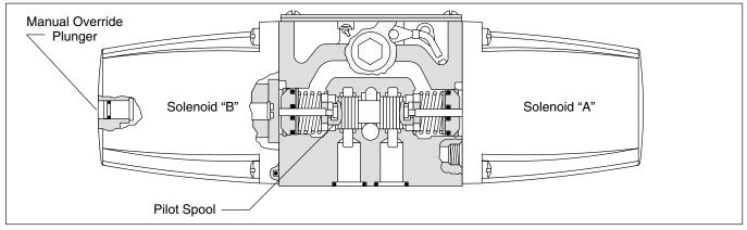
Figure 13c. DG4S4-01-50 Pilot Valve, Sectional View
