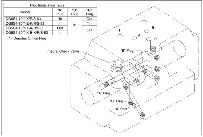
Figure 26b. DG5S4-10\*\*-(K/R/S)-53 Internal Pressure Passages & Plug Locations
