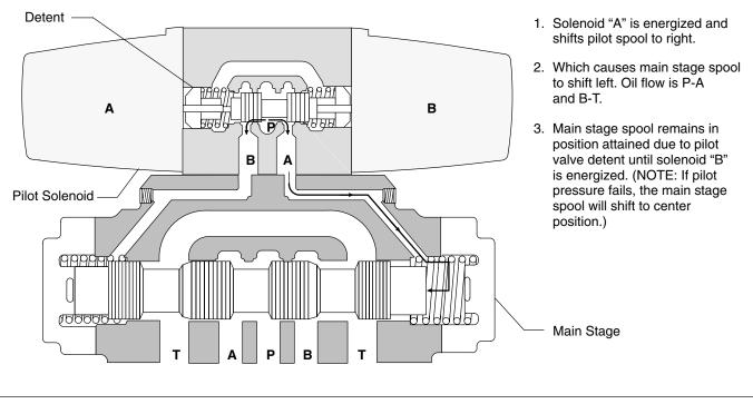
Figure 8. Detented "N" Model
