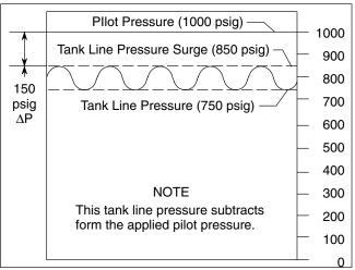
Figure 14. Pilot Valve - Internal Drain
