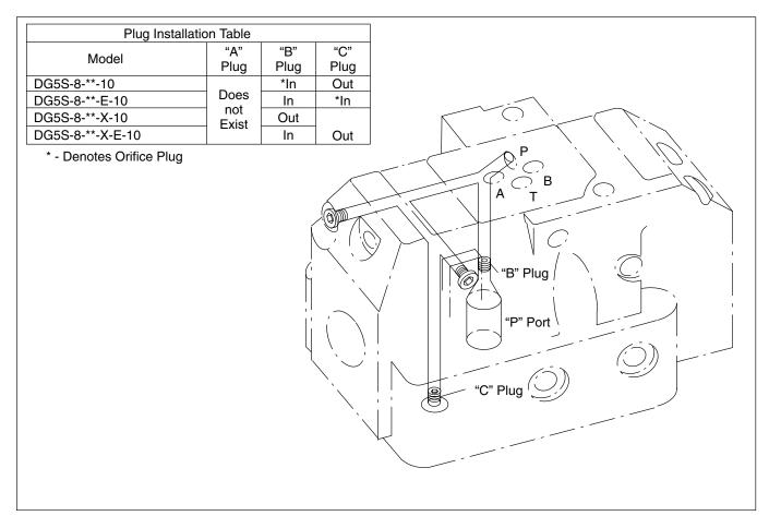
Figure 27a. DG5S-8-\*-10 or DG5S-H8-\*-20 Internal Pressure Passages & Plug Locations
