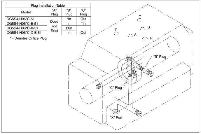
Figure 25a. DG5S4-H06-\*-51 Internal Pressure Passages & Plug Locations
