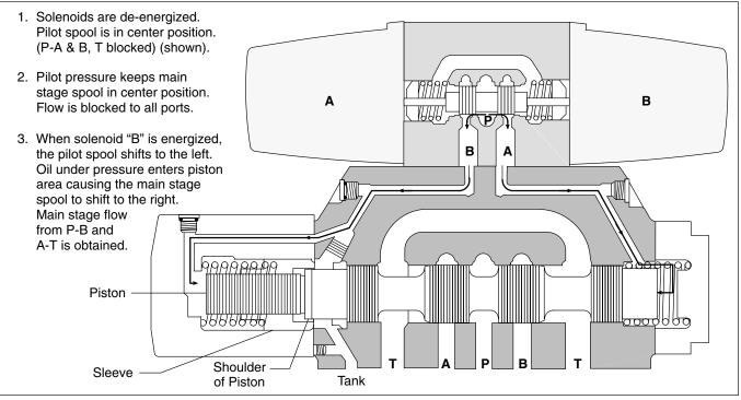
Figure 7. Pressure Centered "D" Model
