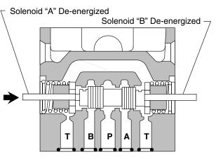
12b. Flow Conditions Pressure to "A" - "B" to Tank
