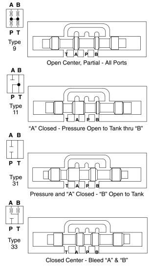
3. **Integral Pilot Valve**: The integral pilot type two stage valve is a very common valve used in the field today. Two stage valves allow large volumes of fluid to be switched to and from an actuator with minimum power required for control. Reference Figures 4 through 8, shown in the following section.
