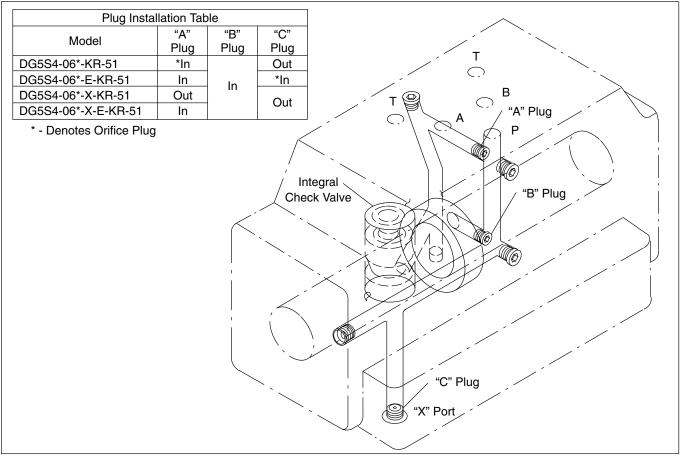
Figure 24b. DG5S4-06\*-(K/R)-51 Internal Pressure Passages & Plug Locations
