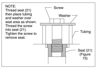
Figure 16. Check Valve Seat Removal
