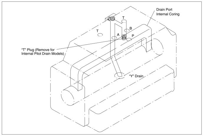
Figure 25c. DG5S4-H06-T-51 Internal Drain Passages & Plug Locations
