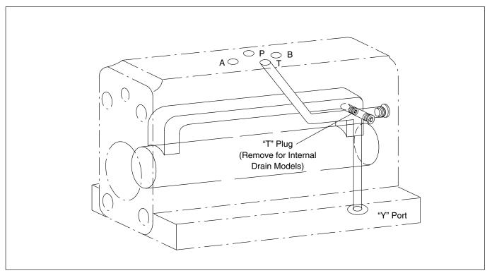
Figure 23c. DG5S4-04-T-40 Internal Pressure Passages & Plug Locations
