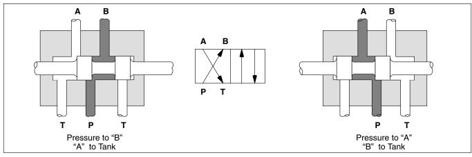
Figure 1. Spool Type Four-Way Valve
