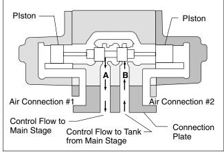
Figure 11b. DG18S4-\*\*-52 Air Operated Pilot Valve
