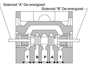
12c. Flow Conditions Blocked (Center Condition #2 Spool)
