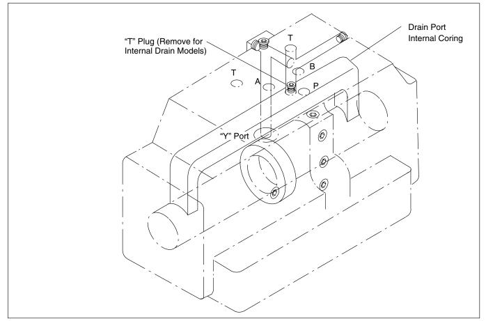
Figure 26c. DG5S4-10\*\*-T-53 Internal Drain Passages & Plug Location
