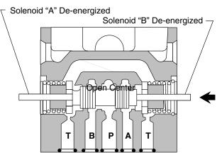
12a. Flow Conditions Pressure to "B" - "A" to Tank
