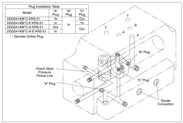
Figure 25b. DG5S4-H06-(K/R/S)-51 Internal Pressure Passages & Plug Locations
