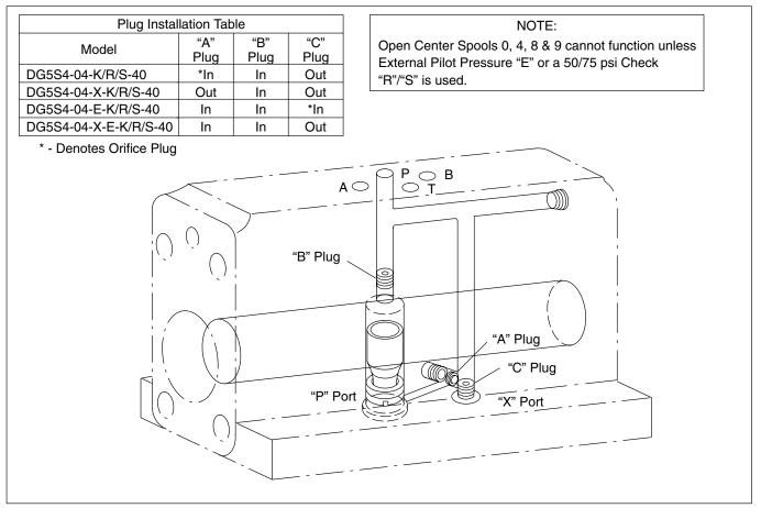
Figure 23b. DG5S4-04-(K/R/S)-40 Internal Pressure Passages & Plug Locations
