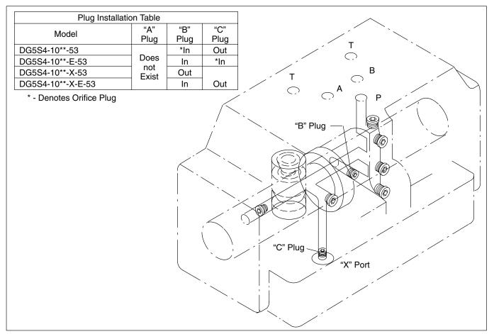
Figure 26a. DG5S4-10\*\*-53/54 Internal Pressure Passages & Plug Locations
