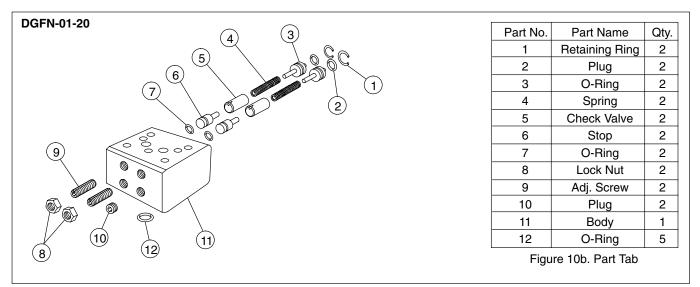
Figure 10b. Pilot Choke - DGFN-01-20 (Use with DG4S4-01 Series)
