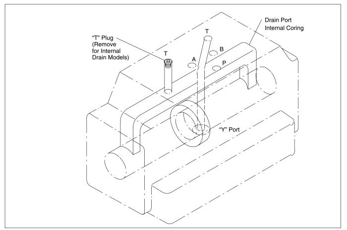
Figure 24c. DG5S4-06-T-51 Internal Drain Passages & Plug Locations
