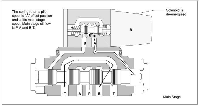
Figure 6. Spring Offset "A" Model
