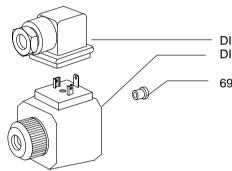
DIN Coil Mating Receptacle DIN Coil (See Table)
